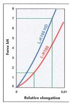
Analyses carried out by well recognised Finnish University are clearly illustrating that the relative elongation of DEWA L-K 160 for a tank dim. 60m x 7m is 0,0035 and for the L-K 160HD with tank dim. 150m x 12m, 0,007 respectively (see left curves)
